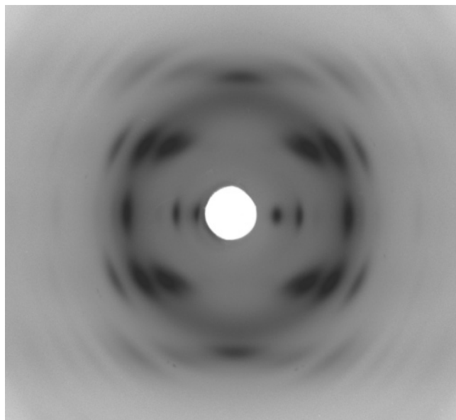
Figure 1. X-ray fiber diffraction pattern of a uniaxially stretched film presenting the s-PS/NB molecular complex phase.
